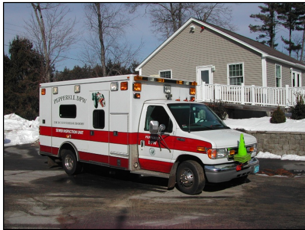
Retrofitted ambulance now serves as Sewer Division CCTV mobile unit.
