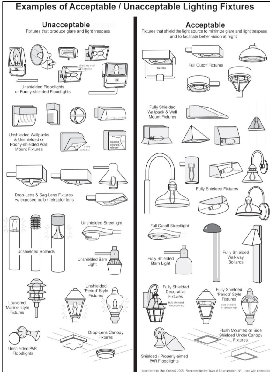
Figure 2: Examples of acceptable and unacceptable lighting fixtures / luminaires. The intent of this figure is to demonstrate that “acceptable” lighting eliminates or reduces glare by hiding the light emitting portion of the bulb or lamp, not that the general style of fixture is prohibited.
